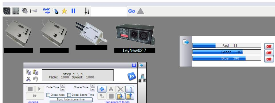
After add and finishing setting up step,press ico (save as) jumps out of the following window fill in the document needing to preserve, at the same time choose “add to cue” frame ,press the button of “save to preserve it ,and then exit.
