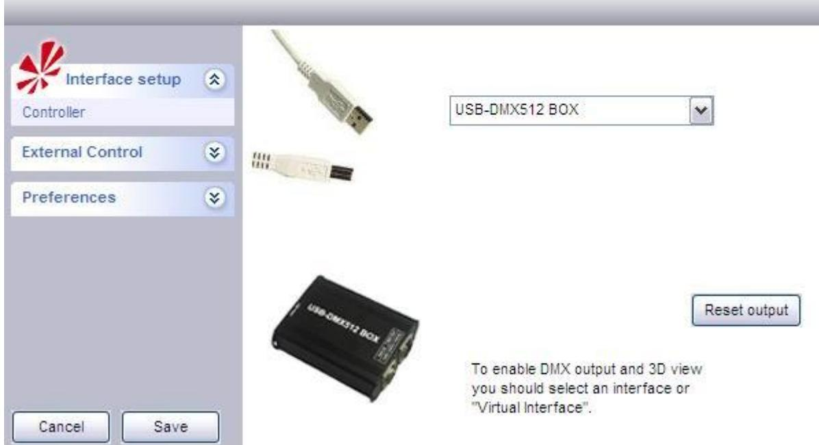
If have chosen DMX interface, and have USB wire to connect DMX interface,such as USB-DMX512 interface,reset FreeStyler software, when schedule bar process to 80%, if the blue LED light of interface bright , means the software recognize the interface, DMX signal could output at this moment.
