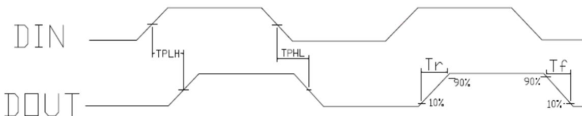
11. The data transmission time ( $T_H+T_L=1.25\mu s\pm 600ns$ ):
