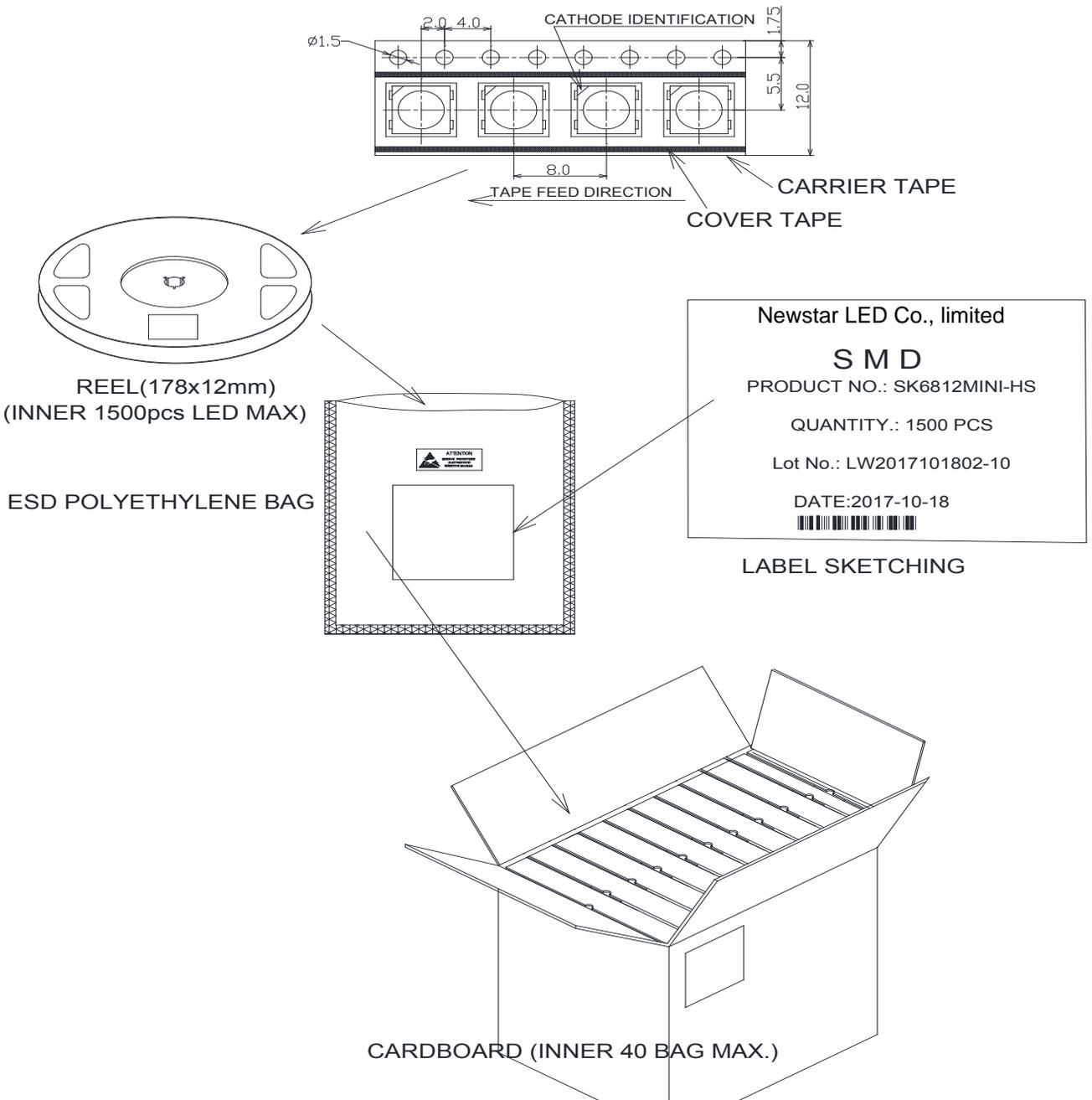
The reel pack is applied in SMD LED. The LEDs are packed in cardboard boxes after packaging in normal or anti-electrostatic bags. cardboard boxes will be used to protect the LEDs from mechanical shocks during transportation. The boxes are not water resistant and therefore must be kept away from water and moisture.
