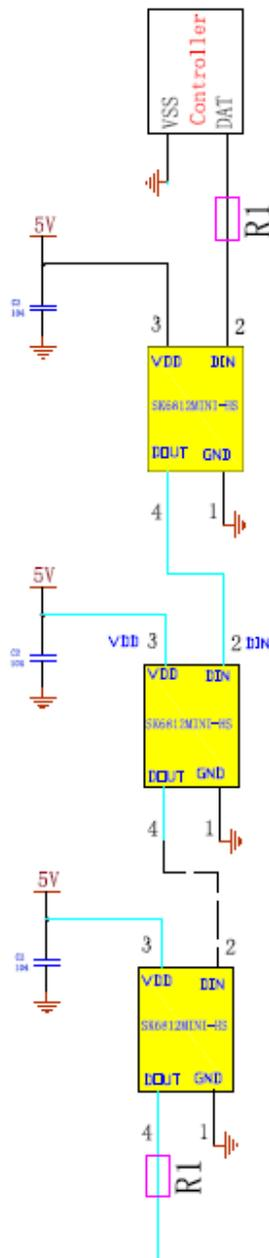
Product signal input and output must be connected in series Protection resistor R1, R1 depends on the size of the cascade lamp beads, the greater the number of cascade, the smaller R1, the general recommended value between 200-2KΩ, usually recommended Worth about 500 euros;
