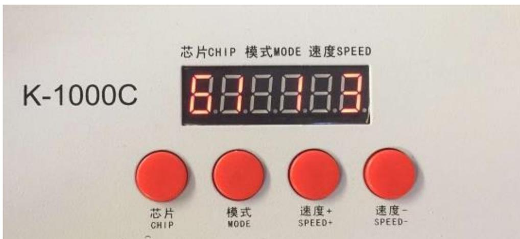
**NOTE:** 61 means UCS512A or B coding mode; 62 means WS2821 coding mode; 63 means SM DMX512AP; 64 means UCS512-C; Ch.: 03 means the coding channel is 3 channels
