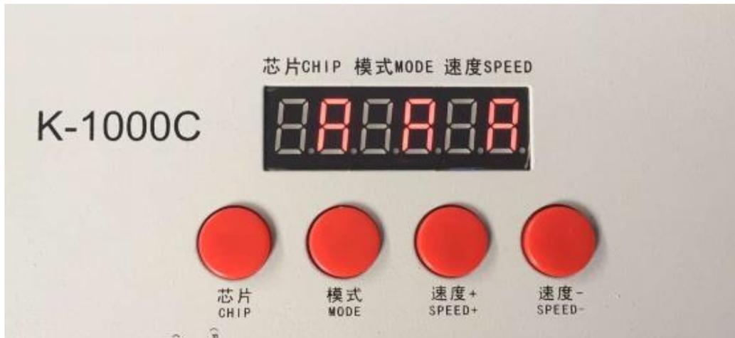
3. After finished address code, press “CHIP” first and at the same time press “MODE” button, switch to playback mode, switch the chip to Chip: 10, this is the DMX512 standard agreement 250Kbps playback mode. At this time, press MODE button and SPEED button can separately switch playback mode and adjust speed, as below:
