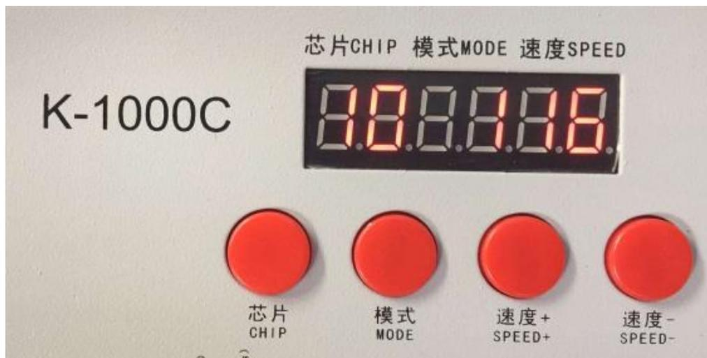
Special Remarks: Derived program after set one-key coding in the software, long press MODE for 5 seconds can write code to the lights directly, this function is very convenient and practical. Welcome to consult our engineer or salesman to learn the detailed operation method.
